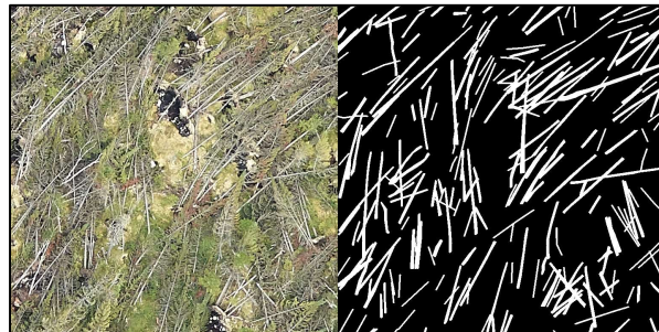
Figure 1. 38.4x38.4m section of aerial image (left) and corresponding manually segmented mask (right)
