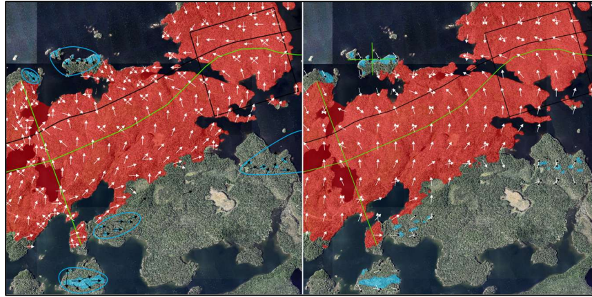
Figure 4. Manual (left) vs. automated (right), Fujita-style treefall direction fields, 4.25x4.25km, 250m grid size
